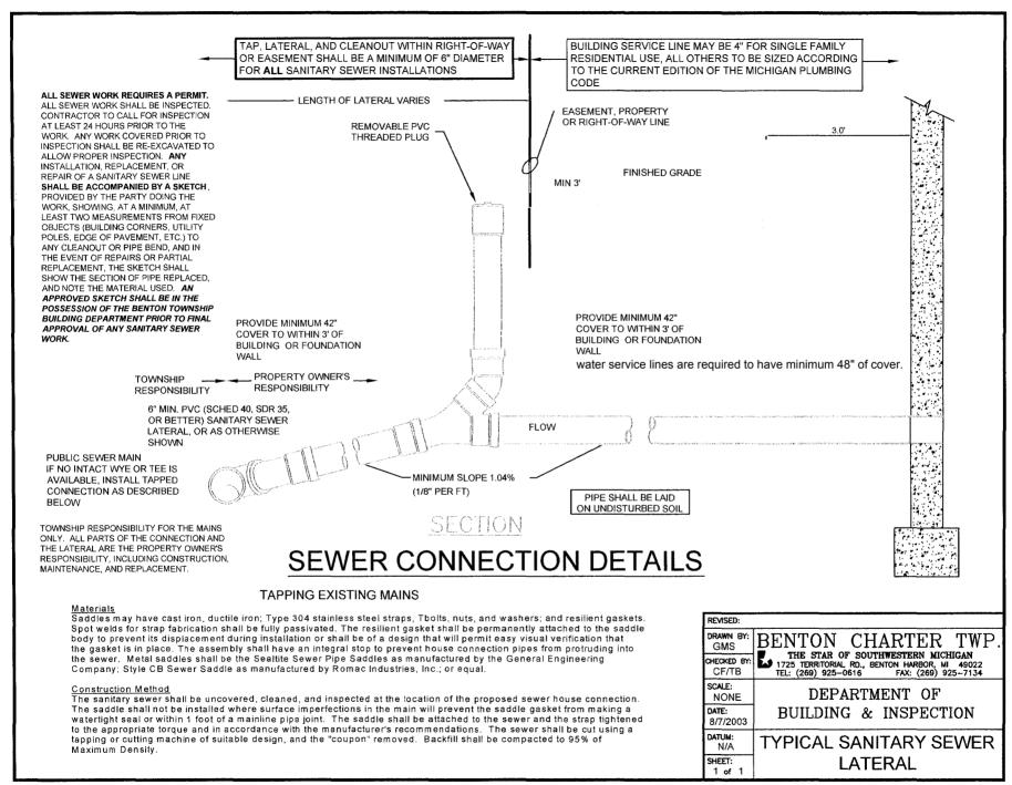
Water lines installed in the same trench shall meet the requirements of the Michigan Plumbing code, Section 603.2 separated from the sewer pipe by 5 (five) feet in the trench, excepting where the water service pipe is 12" above the top of the highest point of the sewer, or where sewer materials are of approved materials, or where the water pipe is sleeved 5' both sides of where the pipes cross in the trench with an approved sleeve. Please call if you have questions.
